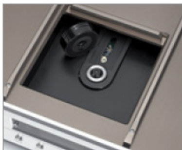
Sliding door and CD "puck" – that takes time. But it does load fast...
