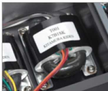
Such transformers produce hardly any relevant stray fields
