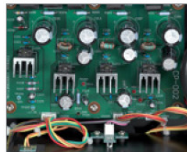
Separate voltage regulators supply the various sections of the transport
