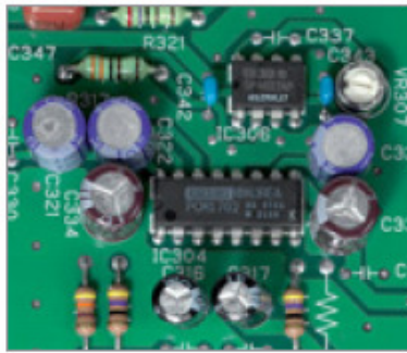
The well-known PCM1702 is used as the digital-to-analog converter
