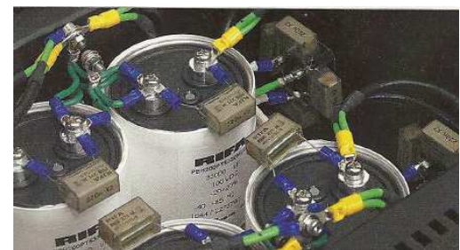
Specially made large capacitors from Rifa
