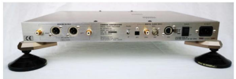
There are four possible digital inputs, both RCA and XLR analog outputs.
